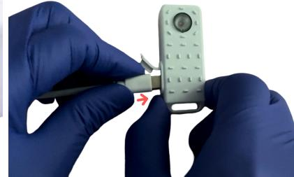
Step 2: Plug charging cable into Firefly.
